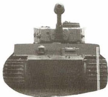
PzKw VI AUSF E — better known as the Tiger; it carried an 8.8cm, KWK 36, L/56 gun.
